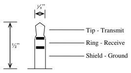
The transmit signal is for data originating at the Tunerone, to be received by the connected device. The receive signal is for data ori<sub>TTL</sub> ing at the connected deviTIA/EIA-232-E y the Tunerone. The circuit for connection to a standard TIA/EIA-232-E connector is as follows:
